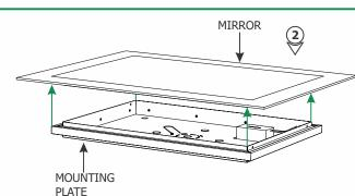
**3:** Align the mounting plate hole with the power line conduit, or junction box. Use the mounting plate as a template to mark four mounting holes (highlighted in GREEN) onto the wall.
