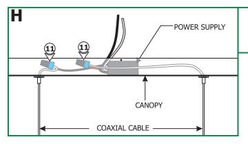
**11:** Connect the bare wire from the +24VDC coaxial cable to the red transformer wire using a wire nut. Connect the bare wire from the -24VDC coaxial cable to the black transformer wire using a wire nut.
