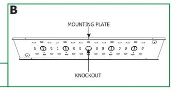
2: Select the appropriate knockout on the mounting plate and remove it using a flathead screwdriver or other appropriate tool
