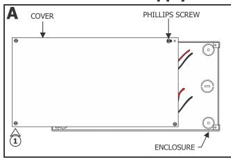
**1:** Loosen the four Phillips screws on the front of the power supply cover to slide the cover off of the enclosure.
