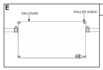
**10:** Replace the power supply cover and secure it by tightening the four Phillips screws.
