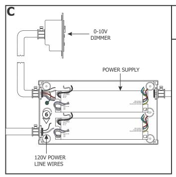
**6:** Run the 120 volt power line wires from the panel to the power supply case.
