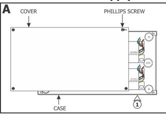
**1:** Loosen the four Phillips screws on the front of the power supply cover to slide the cover off of the case.
