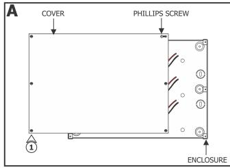
**1:** Loosen the Phillips screws on the front of the power supply to remove the cover.
