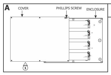
**1:** Loosen the six Phillips screws on the front of the power supply cover to slide the cover off of the enclosure.
