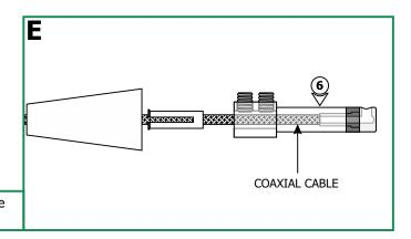
**6:** Feed the coaxial cable into the coaxial fixture connector. The coaxial cable will come to a stop point.
