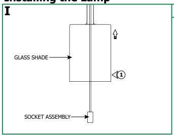
1: Lift the glass shade up to expose the socket assembly.
