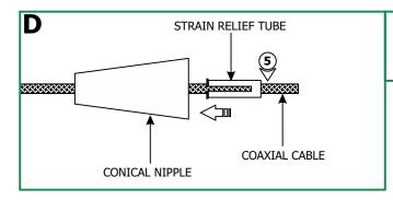
**5:** Feed the coaxial cable through the conical nipple and flared side of the strain relief tube. Slide the conical nipple and strain relief tube down the coaxial cable.
