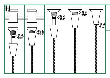
12: Use fingers to tighten the Fast Jack fixture connector into the Fast Jack system connector (Monorail, Monorail Wall, Monorail 2 Circuit, or multi-port and mono-point canopies. Refer to the instructions provided with the system connector or canopy).
