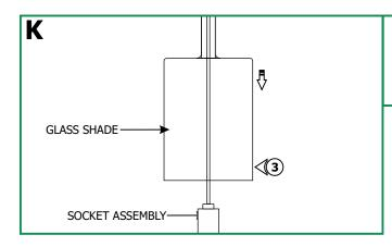
**3:** Carefully lower the glass shade onto the socket assembly.
