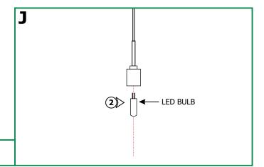
**2:** Insert LED bulb into 2-pronged socket, and re-attach the bottom portion of the fixture
