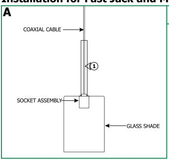
**1:** Feed the coaxial cable through the glass shade, and rest the glass shade over the socket assembly.
