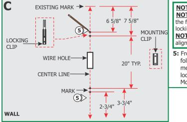
**NOTE:** AV2-IRE is shown for demonstration purposes. **NOTE:** Locking clip must be installed in the opposite direction of the fixture wire. Fixtures greater than 36" are provided with two locking clips. **NOTE:** The junction box could be offset, but needs to be
