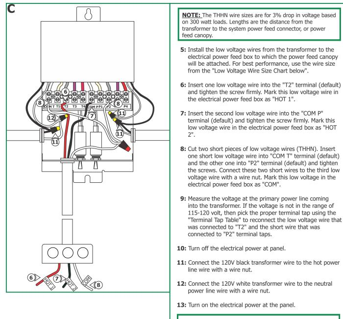
**NOTE: Risk of Fire** - The terminal taps **ARE NOT** for boosting the transformer low voltage power, they are selected to ensure output power voltage based upon input power voltage condition. **NEVER** use a higher terminal tap to compensate for voltage drop, this will overheat the low voltage wires and transformer. It is recommended to use the wire size as indicated in "Low Voltage Wire Size Chart" on page 4 to avoid excessive voltage drop.
