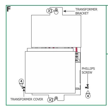
**NOTE:** In order to use small gauge wires from the transformer to the electrical box, it is recommended to install the remote transformers as near as possible to the electrical box. See "Low Voltage Wire Size Chart" located below.
