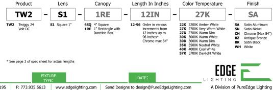
Application: Electronic low voltage dimming for Twiggy S1
