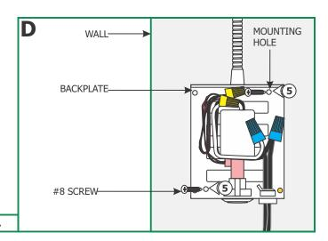
**5:** Mount the backplate to the anchors with the two #8 screws.
