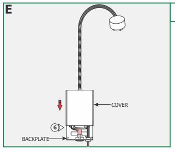
**6:** Replace and slide the cover down completely onto the backplate.
