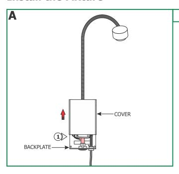
1: Remove the cover by sliding it up and then off the backplate.
