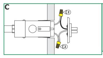
**NOTE:** The low voltage wires should be present in the 2" electrical box. Refer to the instructions provided with the remote transformer to install the transformer and the low voltage wires before proceeding with the steps below.
