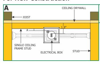
**1:** For Single Ceiling Frame Stud, use the Monorail 2" standoff to mount the Feed-End Power Canopy closest to the ceiling. Refer to the chart below to determine the 2" electrical box distance from the ceiling frame stud.
