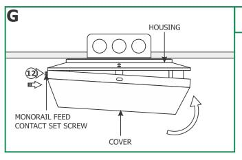
**12:** Hook one of the transformer cover screw holes next to the rectangle cutout, onto the Monorail feed contact set screw.
