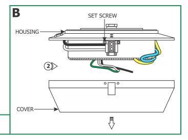
**2:** Unhook the transformer cover from the set screw and remove it from the transformer housing.
