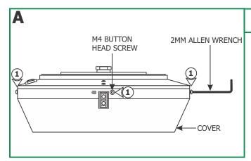
**1:** Loosen and remove the five M4 button head screws around the transformer cover with the provided 2mm Allen wrench.
