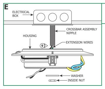
**9:** Feed the extension wires through the transformer housing center hole. Slide the transformer housing onto the crossbar assembly nipple and secure it in place by
