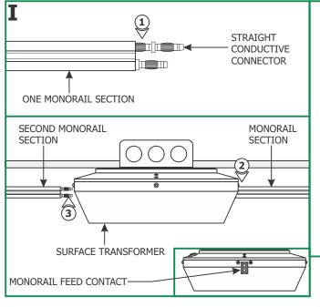
**NOTE:** The Monorail 1" standoffs should be installed before connecting the Monorail to the transformer (refer to the instructions provided with the Monorail 1" standoffs).
