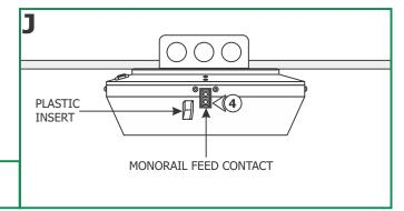
**4:** If using only one Monorail section then plug the unused Monorail feed contact with the plastic insert provided.
