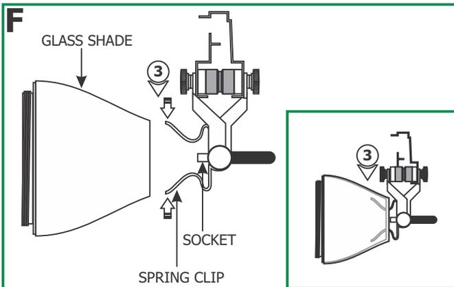
**3:** Squeeze the spring clip ends while inserting it into the glass shade.
