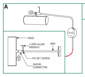
1: Rotate the Cody's head perpendicular to the arm making sure the arm is completely inserted into the head. Tighten the M3 set screw on the swivel connector with the provided 1.5mm Allen wrench to secure the head in place.
