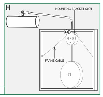
14: Hang the frame cable into the mounting bracket slot.
