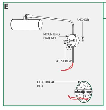
**9:** Line up the mounting bracket holes with the anchors and secure the fixture to the anchors with the two #8 screws provided.
