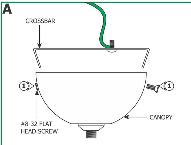
**1:** Loosen and remove the two #8-32 flat head screws from the canopy to remove the crossbar.
