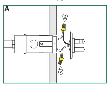
**NOTE:** The low voltage wires should be present in the 2" electrical box. Refer to the instructions provided with the remote transformer to install the transformer and the low voltage wires before proceeding with the steps below.
