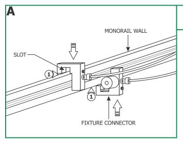
1: Place one fixture connector slot from the top and the other one from the bottom onto the Monorail Wall.
