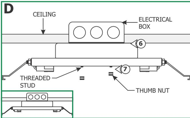
**6:** Place all wires and wire nuts connections inside electrical box.
