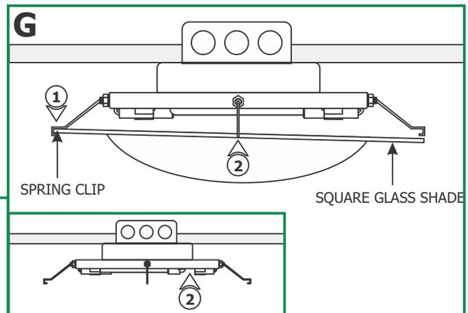
**1:** While holding the glass shade unhook one spring clip at a time until the glass shade is free.
