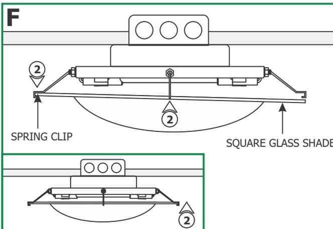
**2:** Place the two adjacent edges of the square glass shade into two adjacent spring clips. Slightly push the glass shade against these two spring clips and simultaneously slide the other two edges into the other two spring clips. **Make sure all four edges of the glass shade sit properly into four spring clips.**
