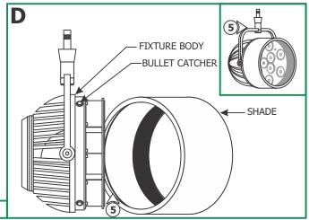
**5:** Snap the inside shade onto fixture body bullet catchers.
