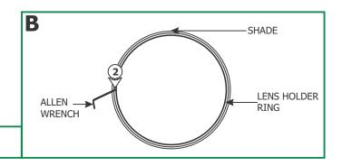
**2:** Use a small Allen wrench or a pen point to loosen and remove the lens holder ring from the shade.
