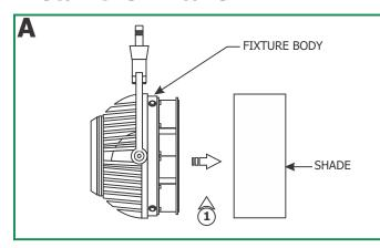
1: Pull the shade out to remove it from the fixture body.
