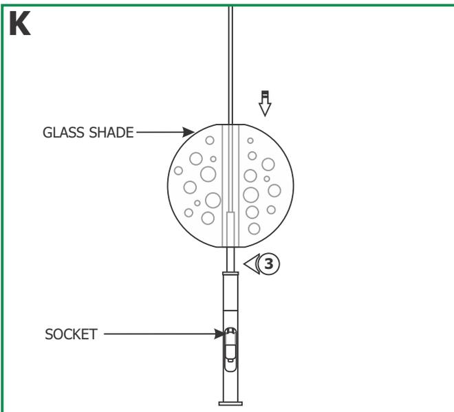
**3:** Carefully lower the glass shade onto the socket assembly.
