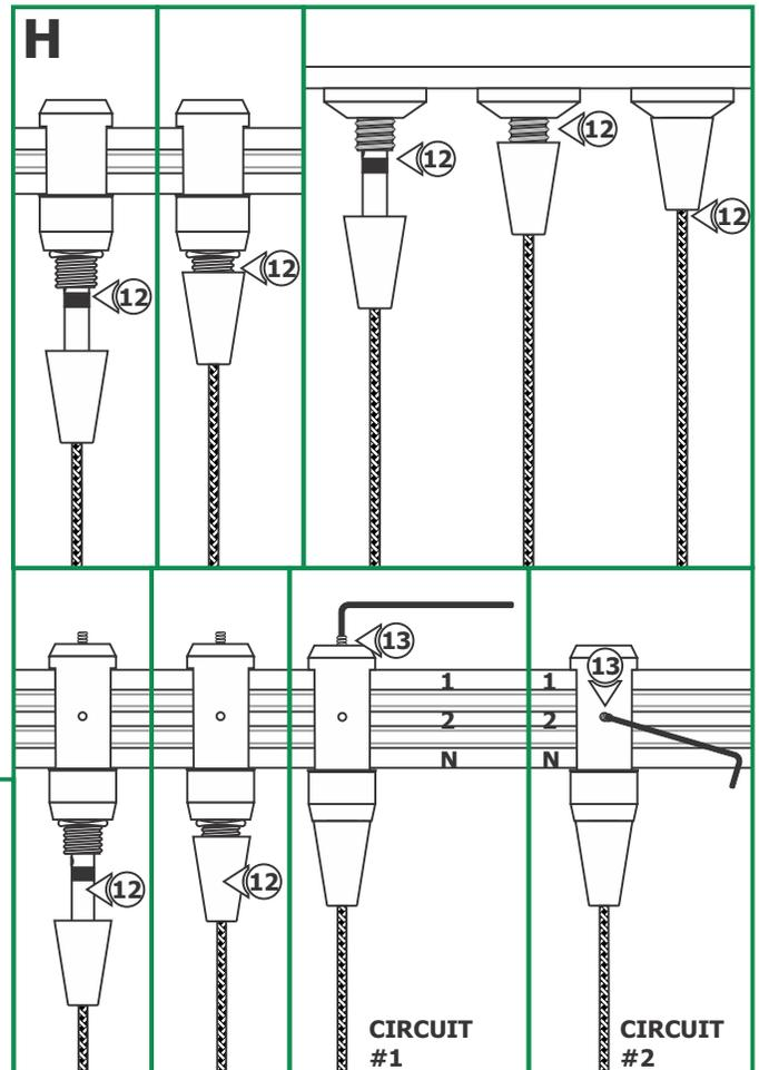
**12:** Use fingers to tighten the Fast Jack fixture connector into the Fast Jack system connector (Monorail, Monorail Wall, Monorail 2 Circuit, or multi-port and mono-point canopies. Refer to the instructions provided with the system connector or canopy).
