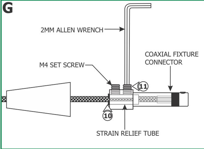
**10:** Push the strain relief tube completely into the coaxial fixture connector. Make sure the slot on the strain relief tube is not inline with the M4 set screw.
