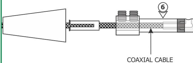
**7:** Keep feeding the coaxial cable in until the inner wire is visible in the screw hole of the fixture connector tip. The outer metal jacket will start to wrinkle.
