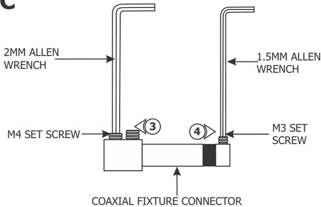
**3:** Loosen the two M4 set screw on base of the coaxial fixture connector with the 2mm Allen wrench provided. **Do not remove these set screws.**
