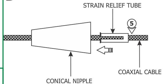
**6:** Feed the coaxial cable into the coaxial fixture connector. The coaxial cable will come to a stop point.
