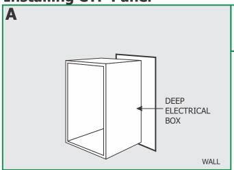
1: On the selected wall, install deep double gang boxes to fit the controller and controller power supply (OT-20-120-240-245 recommended).
