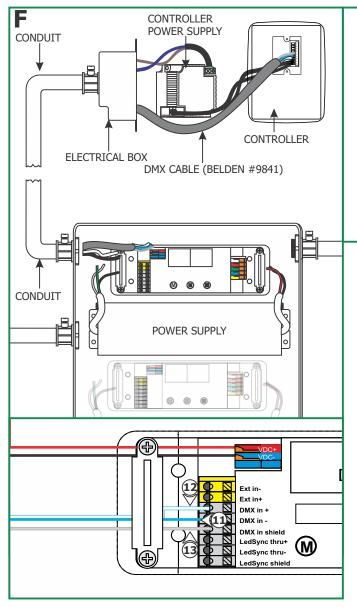
**NOTE:** "DMX in+", "DMX in-", "EXT in+" & "EXT in-", controller terminals are not used on controller.
