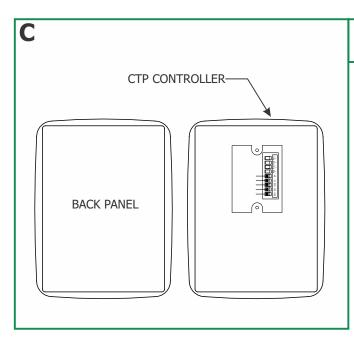
3: Remove the back panel of the CTP controller to attach power supply and DMX controller cables.
