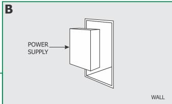
2: On the selected wall, install deep double gang boxes to fit the controller and controller power supply (OT-20-120-240-245 recommended).
