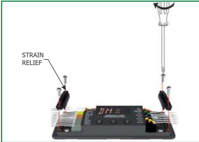
1. On both sides of the DVR-RGB-200, make sure the leads run between the strain reliefs screw holes.
