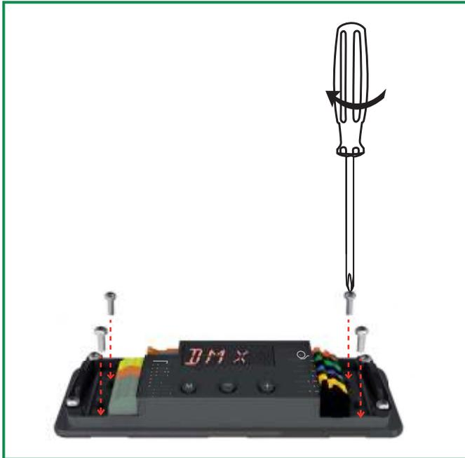
1. The driver/controller has four mounting holes suited for M4 screws. Make sure you have four screws that are appropriate for the surface that you want to mount the driver/controller onto. Use mounting screws with a minimum length of 15mm.
