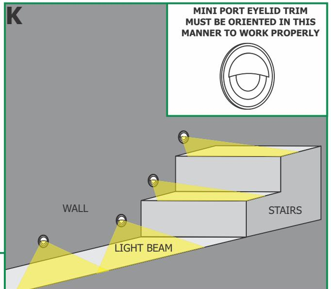
**NOTE:** If installing eyelid Miniport to the walls next to stairs place the trim in the downward position for proper lighting.
