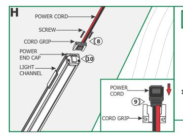
**NOTE:** The power feed cable can be mounted to either the female or male end of the channel.
