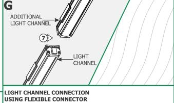
**NOTE:** Multiple light channel can be connected together directly by connecting male end of one to the female end of the other one, or by using the flexible connectors up to a maximum of 10 feet.
