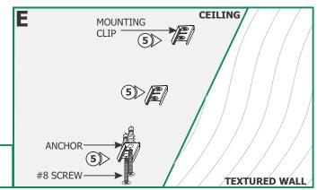
**5:** Line up the mounting clips to the anchors and secure it to the anchors by tightening the two #8 screws to each clip.
