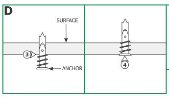
**NOTE:** Steps 3 to 5 are for drywall mounting. Omit these steps if mounting the clips to a wood surface directly. **ANCHORS ARE NOT PROVIDED.**
