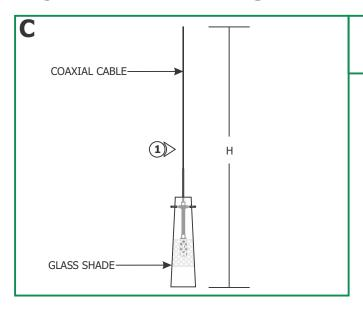
**1:** Cut the coaxial cable to the desired height (H) with a sharp cutter. The overall fixture height is measured from the bottom of the glass shade to the end of the coaxial cable.
