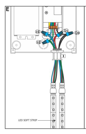
**NOTE:** The DVR-RGB-60 terminals adapt maximum 18 AWG size. To avoid voltage drop, use 6" of 18 AWG size in RGB terminals connected inline to proper size gauge wire attached to the RGB LED wires with wire nuts. See the "Low Voltage Wire Size Chart" on page 1.
