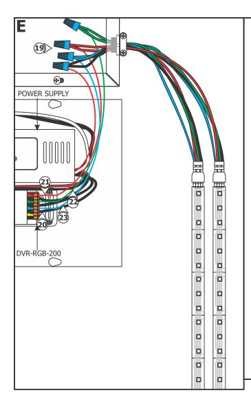
**NOTE:** The DVR-RGB-200 terminals adapt maximum 18 AWG size. To avoid voltage drop, use 6" of 18 AWG size in RGB terminals connected inline to proper size gauge wire attached to the RGB LED wires with wire nuts. See the "Low Voltage Wire Size Chart" on page 1.
