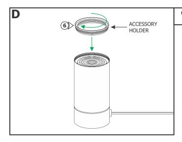
**6:** Screw the accessory holder back clockwise to secure in place.
