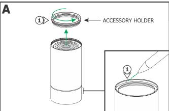
1: Insert a pin such as a pen into the lamp cover and rotate counter-clockwise to remove the accessory holder.
