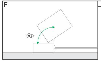
**9:** Adjust the angle of the fixture by rotating the body.
