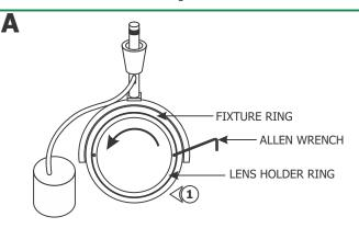
**1:** Use a small Allen wrench or a pen point to loosen and remove the lens holder ring from the fixture ring.
