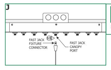
**<u>CAUTION</u>**: **Risk of Fire**: The total load of the Fast Jack canopy ports should not exceed the remote transformer rated capacity.
