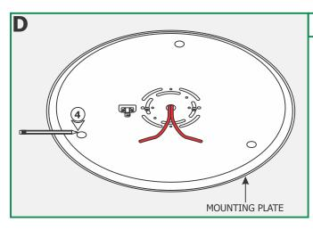
**4:** Mark the three mounting plate holes on the ceiling.
