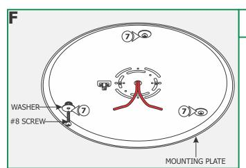
**7:** Secure the mounting plate to the anchors with the provided #8 screws and washers.
