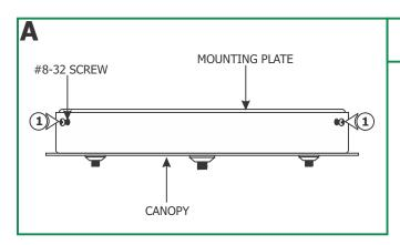
**1:** Loosen and remove the three #8-32 screws from the canopy to remove the mounting plate.
