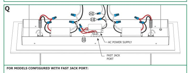
21: Connect the neutral wire from one 120 VAC circuit to the white wire of the AC power supply with a wire nut.
