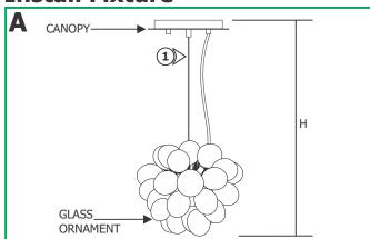
**1:** Determine the desired fixture height (H), from the bottom of the glass ornaments to the top of the canopy.
