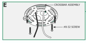
**11:** Mount the crossbar assembly to the electrical box holes with the two #8-32 screws provided.
