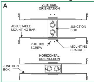
1: Mount each adjustable mounting bar to one side of the junction box (mounts to any side of the housing depending on the orientation of the channel) and secure them with the mounting brackets and two Phillips screws provided.
