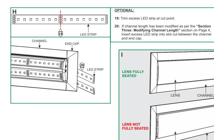
**21:** Snap the lens into the channel and make sure it is fully seated along the length of the channel opening.
