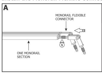
1: Push the Monorail flexible connector pin completely into one Monorail section hole. Make sure this Monorail section is secured with the standoffs (Refer to the instructions provided with the standoffs).
