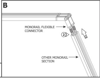
**2:** Push the other Monorail section completely onto the Monorail flexible connector pins and simultaneously connect this Monorail to the standoffs.
