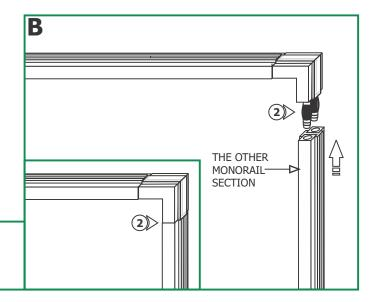
2: Push the other Monorail section completely onto the Monorail ceiling "L" connector pins and simultaneously connect the Monorail to the standoffs.
