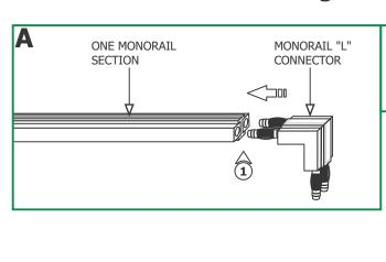
1: Push the Monorail ceiling "L" connector pins completely into one Monorail section. Make sure this Monorail section is secured with the standoffs (Refer to the instructions provided with the standoffs).
