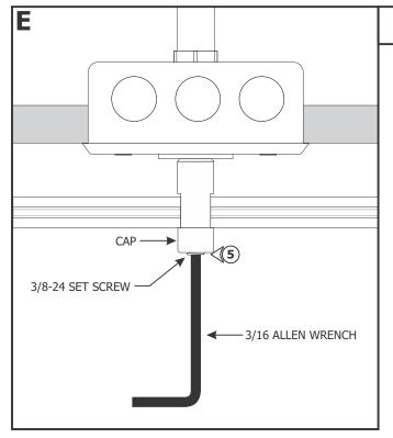
**5:** Tighten the 3/8-24 set screw on the cap firmly with the 3/16 Allen wrench provided for proper power connection.
