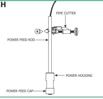
4: Use a pipe cutter to cut out the excess rod. If cutting with a hacksaw, then make sure the center wire is removed from the rod. To remove the center wire, remove the power feed cap, pull the wire out. Make sure to clean the burr of the cut section before re-feeding the center wire.
