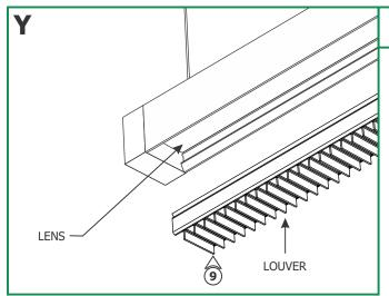
**9:** Install the optional louver to complete the channel assembly by pushing onto the channel over the lens.
