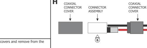
**6:** Unscrew the coaxial connector covers and remove from the connector assembly.
