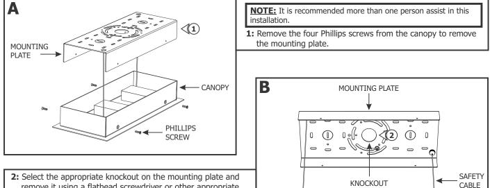
remove it using a flathead screwdriver or other appropriate tool.
