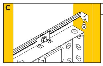
**4:** Screw spacer bars to studs, ensuring that the front face plate stays flush with wall.
