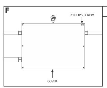
**19:** Replace the power supply cover and secure it by tightening the six Phillips screws.
