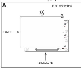
**1:** Remove the six Phillips screws to slide the cover off of the enclosure.
