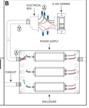
**NOTE:** Refer to wiring diagrams on page 4. Steps 2 through 13 show typical installation for 0-10V dimmers.
