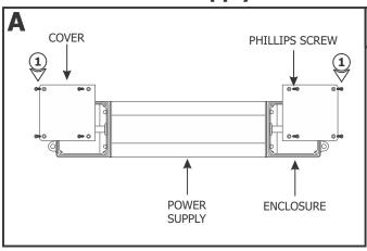
**1:** Remove the four Phillips screws on each cover to remove them from the enclosures.
