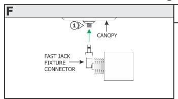
**1:** Use fingers to tighten the Fast Jack fixture connector into the Fast Jack Canopy connector.
