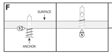
**NOTE:** Omit step 5 if installing to a wood surface.
