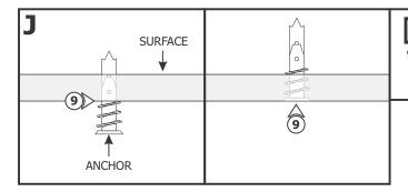
**NOTE:** Omit step 9 if installing to a wood surface.
