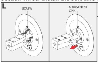
**1:** Loosen **(Do Not Remove)** the four Phillips screws on the adjustment link of each turnbuckle and pull the turnbuckle with the adjustment link out for maximum adjustments.
