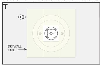
**1:** Apply drywall tape (Ultra-Thin drywall tape suggested) along edges of turnbuckle back plate to prevent cracking of plaster. **Do Not** overlap strips of drywall tape.
