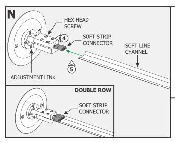
3: Cut the Soft Line channel to determined length.
