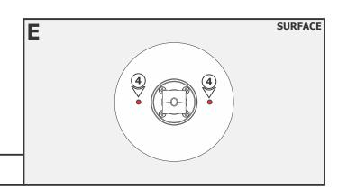
**4:** Place the turnbuckle against the surface and mark the two screw holes.
