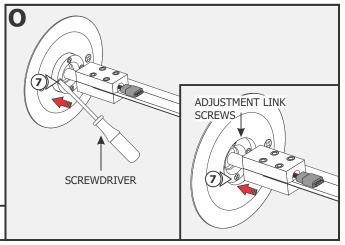
**7:** Tighten the four phillips screws on each adjustment link for the Soft Line channel to stay taut.
