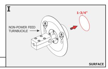
**8:** Place the turnbuckle into the hole and mark the two screw holes.
