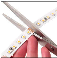
Cut in middle of joining contacts
