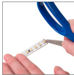
Scrape protective coating from contacts
