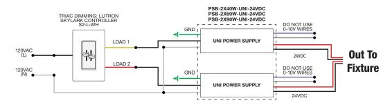
**Application:** ELV dimming for Static White and Warm Dim
