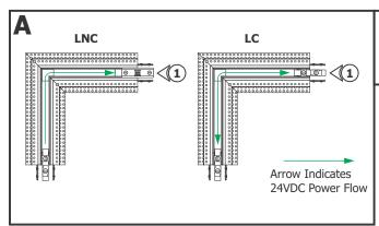
1: L-Connectors join two track sections together in a 90 degree angle and either isolate the power from one track to the other (LNC) or conduct the power from one track to the other (LC).
