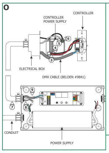
**NOTE:** Use a deep double gang boxes to fit the controller and controller power supply.
