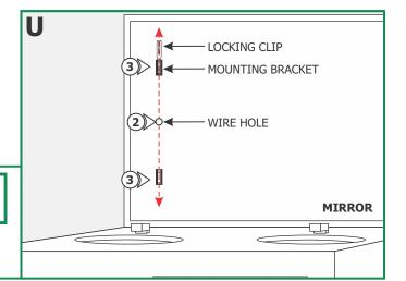
**NOTE:** Locking clip must be installed in the opposite direction of the fixture wire. Fixtures greater than 36" are provided with multiple locking clips.
