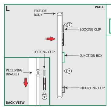
7: Carefully snap fixture body onto the locking & mounting clip(s) then slide into receiving bracket to lock in place. Make sure not to nick the wires.
