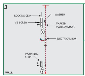
**5:** Secure the locking clip(s) & mounting clip(s) to the marked surface or anchors by passing the screws through the clip holes followed by the washers into the marked points or anchors. Locking clips mount onto mounting clips.
