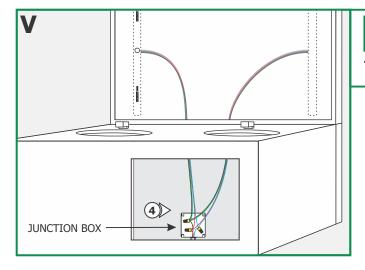
**NOTE:** (Optional) Junction box can be omitted for special installations or where permitted by local electrical code.
