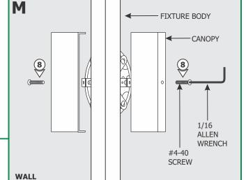
**8 (OPTIONAL):** For 4" Square Canopy installations, place each canopy piece against the crossbar and secure it to the electrical box holes with the provided #4-40 screws using the 1/16 Allen wrench.
