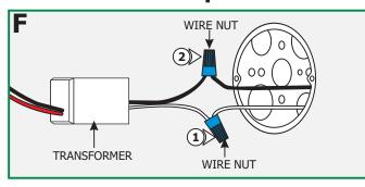
**NOTE:** Low-voltage power wires should be present in the junction box before completing the steps in this section.
