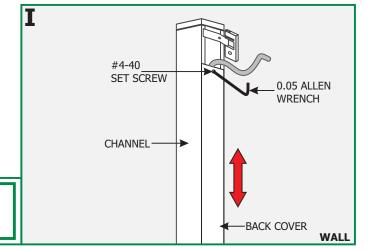
**NOTE:** If the junction box is located at one end of the channel, then loosen the #4-40 set screw with the 0.05 Allen wrench on one of the back cover moving the opening hole to one end. Pull the wire out of that end & retighten the #4-40 set screw with the 0.05 Allen wrench.
