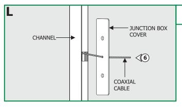
**6:** Pull the coaxial cable through center hole of junction box cover.
