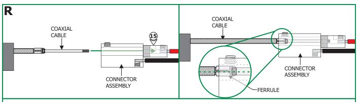
**15:** Insert the coaxial cable into the coaxial connector until the wires of the center conductor are visible through the M3 set screw hole.
