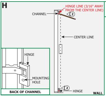
2: Unfold the channel hinges. Align the channel between the marked lines and mark the hinge holes 3/16" away from the center line.
