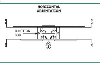
1: Mount each adjustable mounting bar to one side of the junction box (mounts to any side of the housing depending on the orientation of the channel) and secure them with the mounting brackets and two Phillips screws provided.
