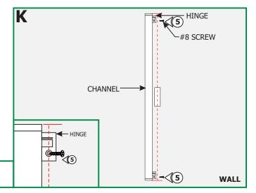
**5:** Line up the hinge to the anchors and secure it by tightening the #8 screws to each hinge.
