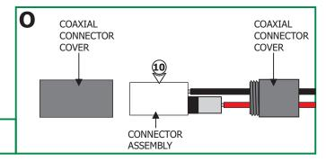
**10:** Unscrew the coaxial connector covers and remove from the connector assembly.
