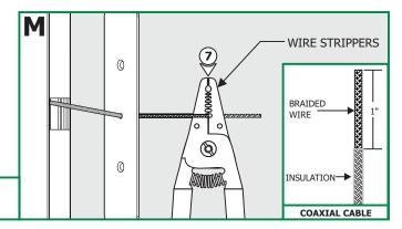
**7:** Using the 16 AWG hole of a pair of wire strippers, remove 1" of outer plastic insulation from the coaxial cable.
